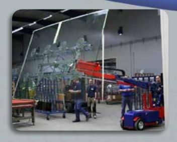
Like its sister model the MAVLift 3080, the smaller MAVLift 2200 is built for serious lifting, transporting, and setting of commercial or specialty glass and materials.
